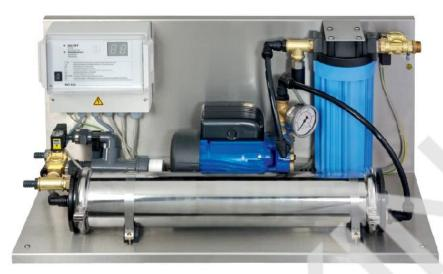
**Under sink or bench unit** for the desalination of softened drinking water (free chlorine not detectable), operating using reverse osmosis (RO). Drinking water can also be desalinated without pre-treatment. However, in this case the recovery rate is reduced. The decisive factor is the water analysis.
